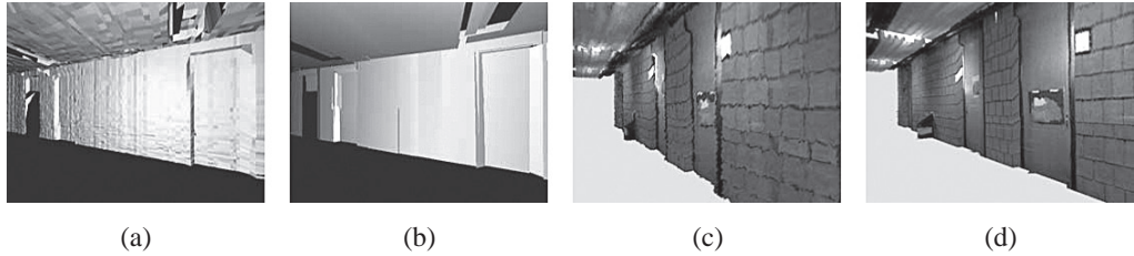
Figure 19.D.1 — Sample results from EM-based 3D plane mapping (a) Raw data map obtained from range finder. (b) Planes extracted from map using EM. (c) Fragment of reconstructed surface using raw data. (d) The same fragment reconstructed using planes.
