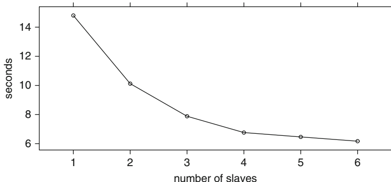
Fig. 5.2 Performance of the Grow–Shrink algorithm for different numbers of slave processes, measured by its execution time (in seconds)
