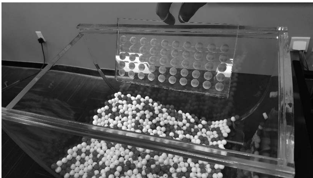
FIGURE 7.2: Inserting a shovel into the bowl.
